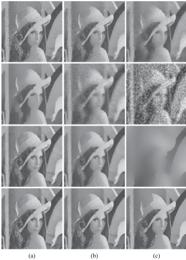
Fig. 8. Results for Lena image with mixture noise in Fig. 6(a) filtered by (from top to bottom) AD, RAD, AMD, and RSF. An evolution step size \tau is set to (a) 0.25, (b) 0.50, and (c) 1.00, respectively. The parameters are the same as those in Fig. 7, except that the number of iterations is 500 and the edge-stopping function in (11) is used, whose potential function is nonconvex. Please see the electronic version for better visibility.
