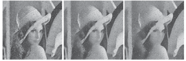
Fig. 11. Behavior of the bilateral filter for the Lena image with mixture noise in Fig. 6(a). The number of iterations is set to (from left to right) 1, 5, and 10. The Gaussian kernel with a size 11 \times 11 is used. The bandwidth parameter is set to the standard deviation of the AWGN, 20. Please see the electronic version for better visibility.
