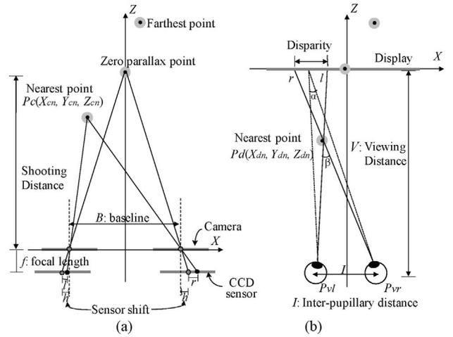
Fig. 1. Geometry of a stereoscopic system. (a) Camera. (b) Display coordinates.
